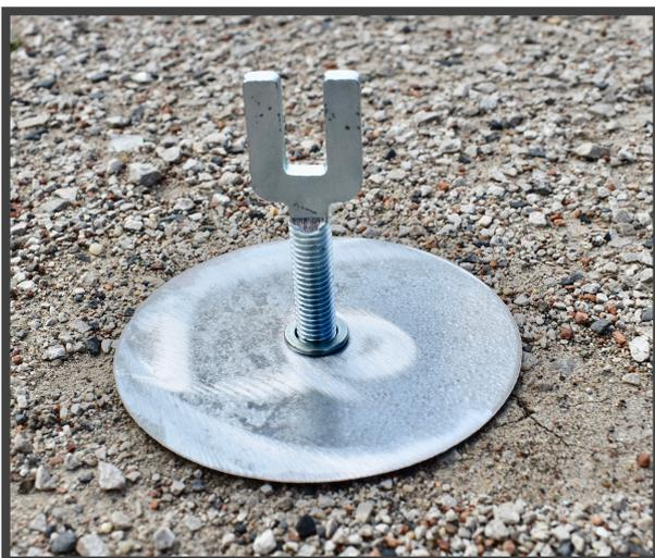
The Blinding Plate shown right is used by knocking a small hole into the sub base which gives your adjustment range, as the blinding is not a structural part of the concrete knocking the blinding plate into the sub base should not cause any problems.
