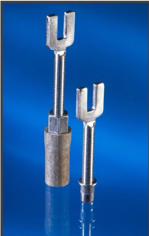
There are two plugs as shown in the image to the left. The small plug is used for depths up to 75mm and the large plug for slabs of greater depths above 75mm. A hole is drilled into the existing concrete and we suggest spacings are 1 meter apart. The small plug requires a 12mm hole and the large plug a 22mm diameter hole. The depth of the whole drilled determines the adjustment range during set up.
